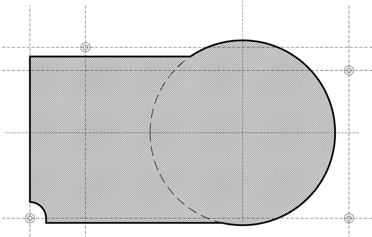
Cutting template and mounting holes for ATX power supply
